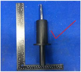
Note 2: With detachable parts removed, if dangerous moving parts of the blender can be touched with the test probe, interlock switch is required on the products to ensure the cutting blade cannot be operated.
